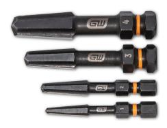
The revolutionary Bolt Biter Screw Extractors use patented tapered sides so the tool sits easily and safely into damaged screws, while the side- and tip-cutting edges provide powerful and consistent extraction. The bi-directional design makes it easy to remove fasteners from the extractor after use but also allows for fasteners to be retightened in an emergency, if need be.
